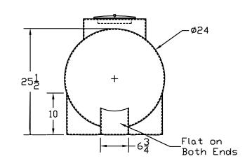
ALL DIMENSIONS SHOWN ARE OUTSIDE PART DIMENSIONS IN INCHES, AND VARY BY THE STANDARD ROTATIONAL MOLDING TOLERANCE OF 2% 10 3%.
