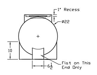
ALL DIMENSIONS SHOWN ARE OUTSIDE PART DIMENSIONS IN INCHES, AND VARY BY THE STANDARD ROTATIONAL MOLDING TOLERANCE OF 2% TO 3%.
