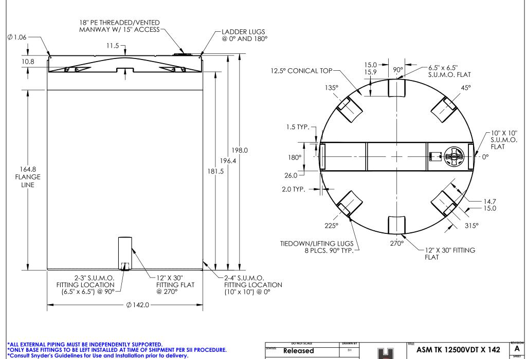
Available on-line at ALL DIMENSIONS ARE IN INCHES, NOMINAL, & SUBJECT TO CHANGE WITHOUT NOTICE. ALL DIMENSIONS ON ROTATIONAL MOLDED PARTS ARE SUBJECT TO A  $\pm$  3% TOLERANCE. HPTC-53500-SI
