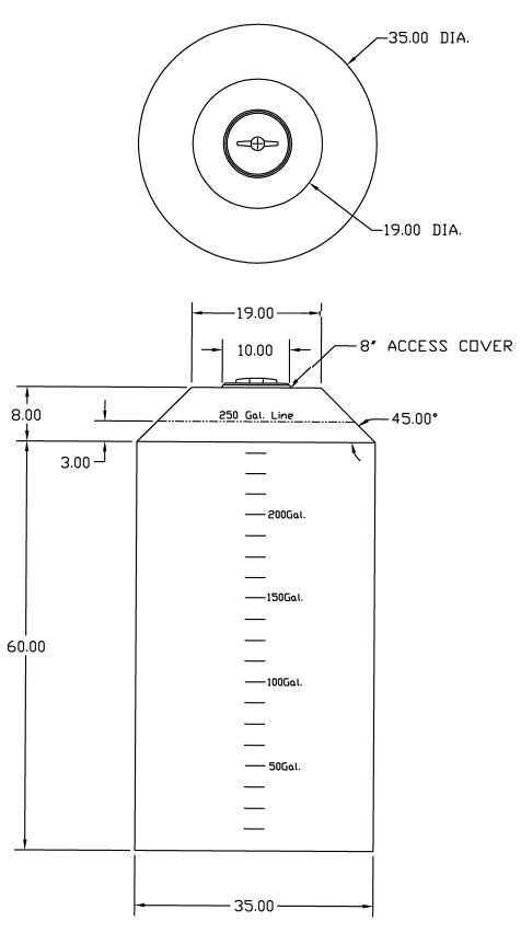
ALL DIMENSIONS SHOWN ARE OUTSIDE PART DIMENSIONS IN INCHESAND VARY BY THE STANDARD ROTATIONAL MOLDING TOLERANCE OF 2% 10 3%.
