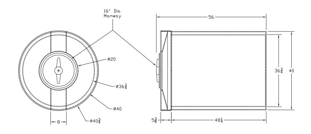
ALL DIMENSIONS SHOWN ARE OUTSIDE PART DIMENSIONS IN INCHES,AND VARY BY THE STANDARD ROTATIONAL MOLDING TOLERANCE OF 2% TO 3%.
