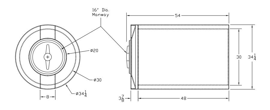
ALL DIMENSIONS SHOWN ARE OUTSIDE PART DIMENSIONS IN INCHES,AND VARY BY THE STANDARD ROTATIONAL MOLDING TOLERANCE OF 2% TO 3%
